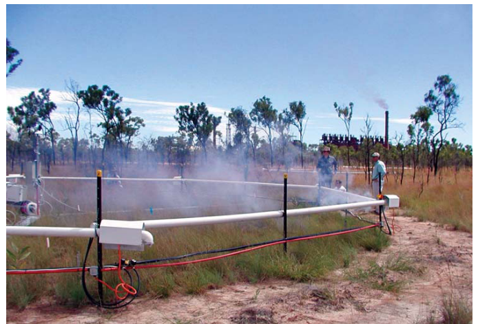
Testing the CO 2 delivery system with a smoke generator during the OzFace installation.
