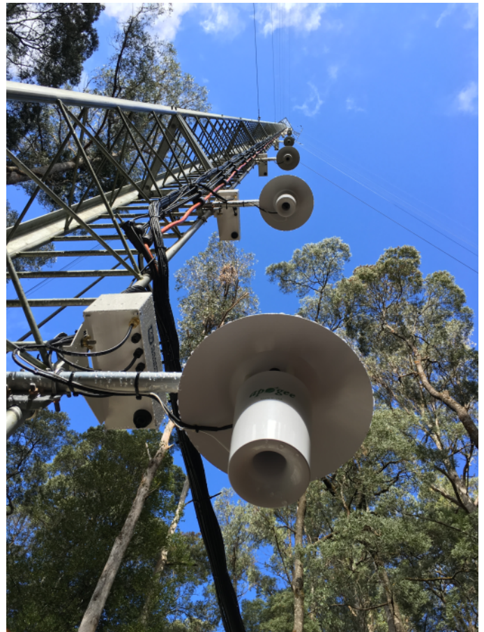
AP200 intakes and temperature probes on the Warra flux tower
