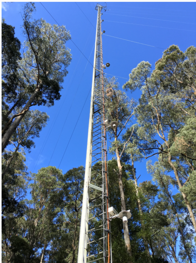
Looking up at the Warra Flux Tower. Several of the AP200 intakes can be seen. The CPEC200 is mounted at the top.
