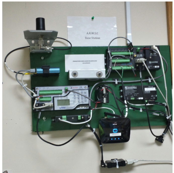
In-office base station tasked with disseminating data and alarms via a synthesized-voice telephone modem and the Internet over cellular and Ethernet, including email and text message
