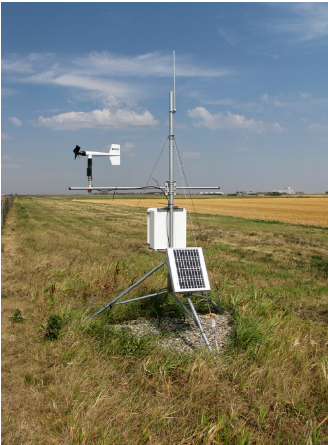
Automated weather stations in Southern Alberta provide real-time wind speed and direction data to local crop dusting pilots
